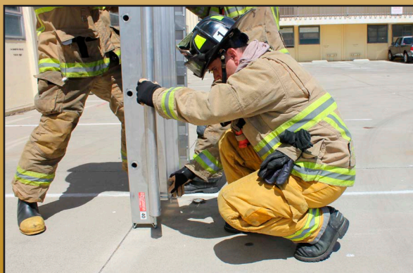
Remove the pin holding the "pike" while the other FF's stabilize the vertical ladder
