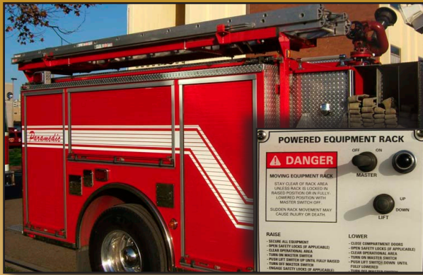
Ladders mounted on top of the apparatus are lowered via a control switch (Inset)
