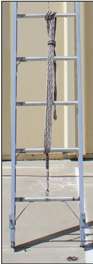
Figure 19-1 Tie-off excess halyard with several wraps around the rungs and secure with a half hitch.
