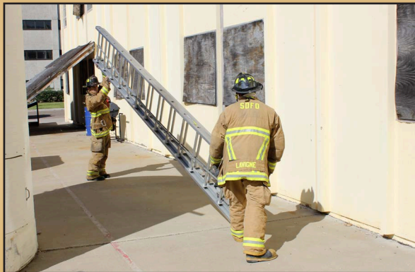
For ladders 28' and larger, someone will need to foot your ladder as you raise it
