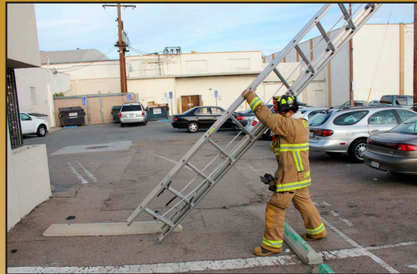
Stick the spurs to your spot and in one smooth motion push up and forward
