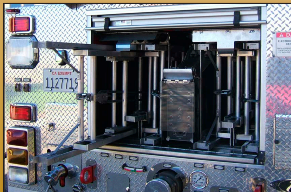
Vertical Racked, Rear Mounted Ladders (Truck Company)
