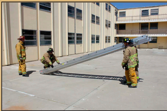
Lower the butt of the ladder to the ground and properly "foot" it
