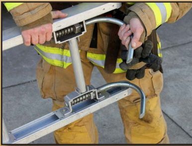
Hooks (Roof Ladder)
