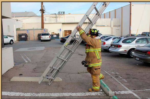
As you push forward on the beam, allow the ladder to pivot on the spur towards you
