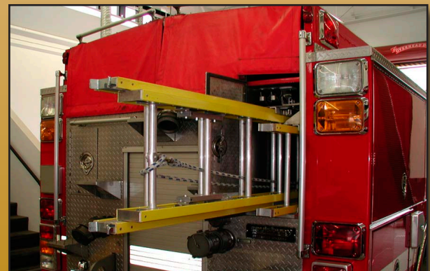
Vertical Racked, Rear Mounted Ladders (Engine Company)
